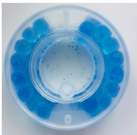
FIGURE 2 Left: Blue sodium alginate (SA) beads are formed directly into the ClinoReactor. ClinoReactor contains 60 sodium alginate beads colored with E133. The gel tip shows how alginate/cell suspension should be dotted into crosslinking solution. Right: Column chart displaying the size of 1% sodium alginate (SA) beads at different days during culture in the ClinoStar system (n =3 in each group).
