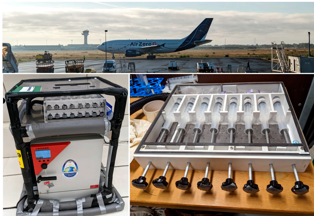
Figure 2. Impressions of the 41st DLR parabolic flight campaign in September 2023, Bordeaux, France. The Airbus A310 Zero G aircraft of Novespace ( top ), the flight rack of the “Thyroid” mission ( bottom left ) and its RNAlater injection system ( bottom right ) are shown.
